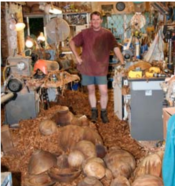
Some of the wood is wet turned as a rough blank for drying. The blank once dry is then remounted on the lathe for finishing. This process can take years depending on the type of wood.
