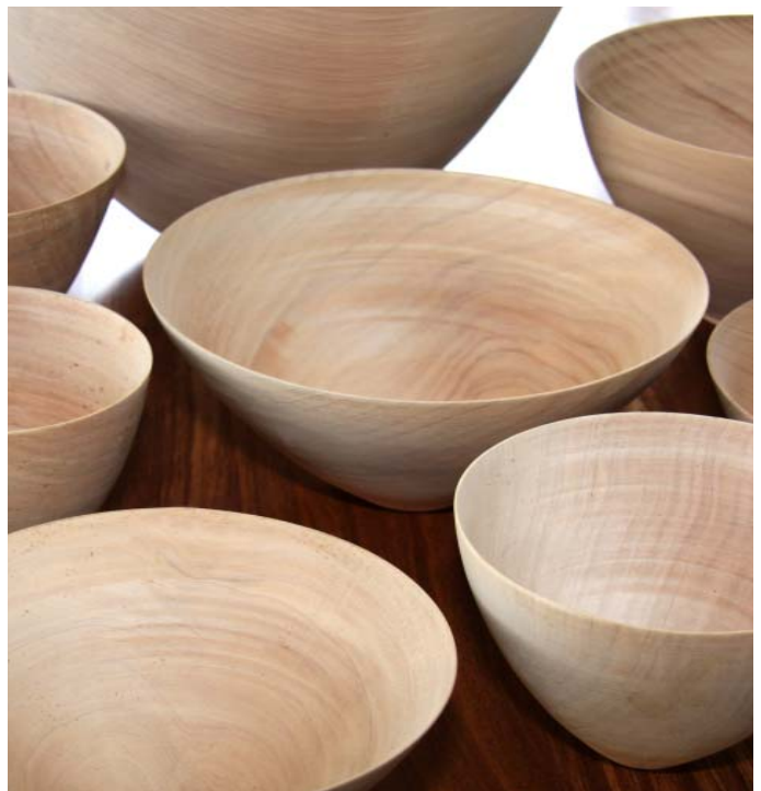
Typically I turn the macrocarpa for my thin vessels when it is wet. The vessels in this picture are all turned from macrocarpa, being only about one millimetre thick they dry quite quickly.
