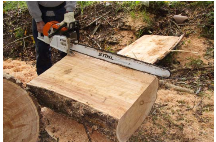
Each piece of macrocarpa is carefully cut with grain orientation in mind for the final piece.
